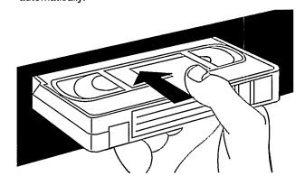
Inserting a cassette will switch on the video recorder automatically. The symbol appears on the display.
